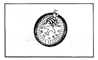
For Pete's sake, set your altimeter. Remember, a one inch decrease in barometric pressure means your altimeter reading is about one thousand feet higher than your actual altitude.
